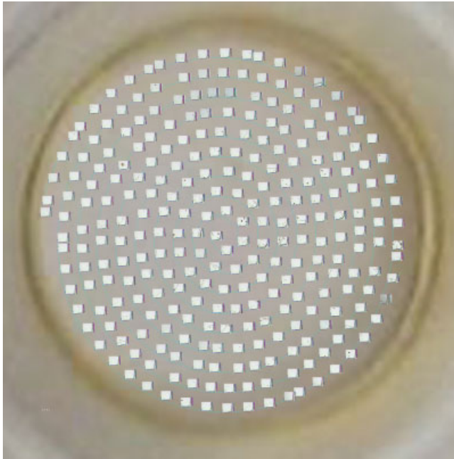
Fig. 1. Uthermöhl chamber with overlaid scanned images and scanning path.
